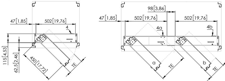
Swing frame mounting option for 800 mm wide cabinets, lateral installation
