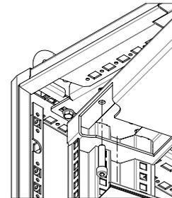
**Swing frame assembly in 800 mm wide cabinets with swing set type 165° type 0318-7080-18-07**
