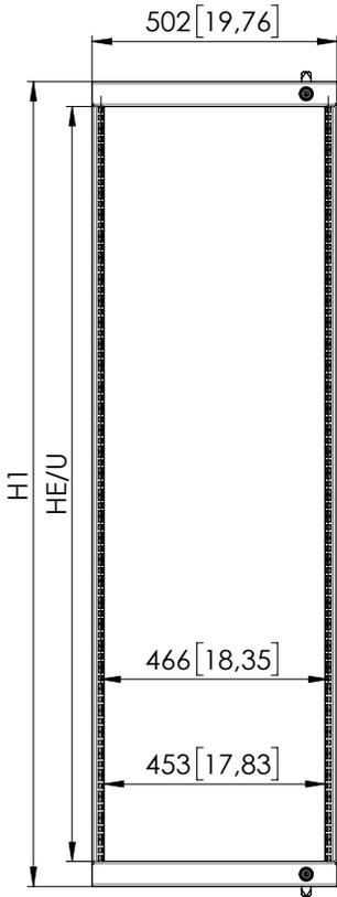
Swing frame for 800 mm wide cabinets, lateral installation
