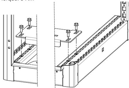
**Swing frame assembly in 600 mm and 800 mm wide**
